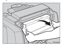
Move the light blue charger cleaner left and right about ten times, and return it to the left side. Align the arrow on the charger cleaner to the arrow on the photoconductor unit.
